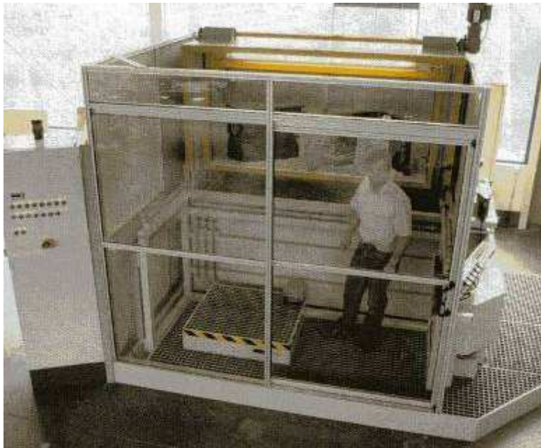
Semi-automated Washout Station
