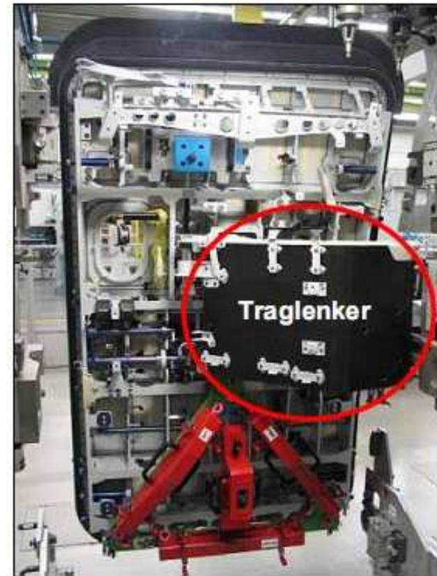
Hinge Arm assembled at Aircraft Door
